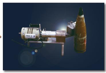
An INL-designed PINS system examines a rusted munition for explosive and chemical signatures.
